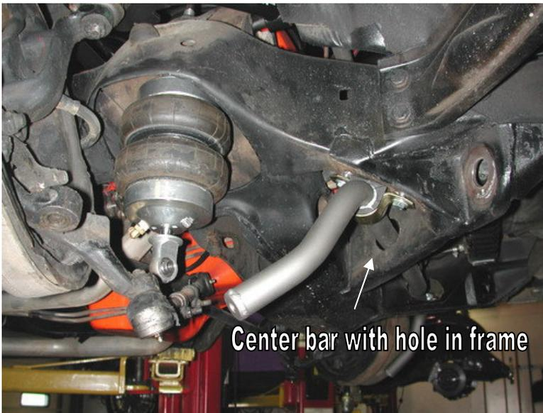
1. Slide the sway bar through the same holes in the frame that the factory bar went through.
