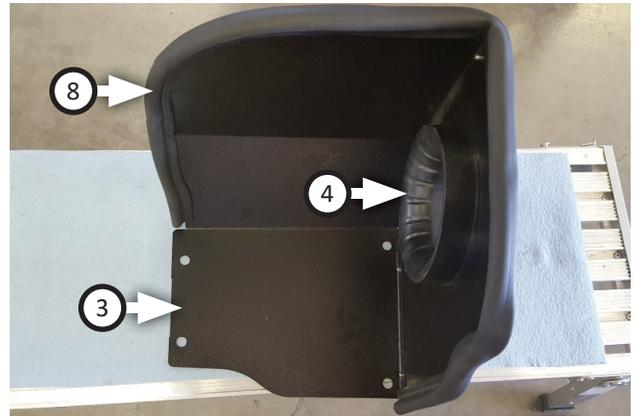
10. Install air filter adapter (4) into airbox (3) using (x3 ea.) screws (13), split lock washers (14) and flat washers (15). Apply trim seal (8) to airbox then trim excess so it fits precisely as shown.
