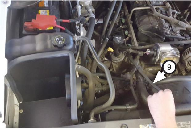
18. Set (x2) **pinch clamps (17)** onto **fuel hose (9)** then install one end onto crank case vent and move pinch clamp over connection.
