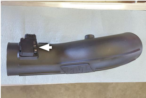
13. Install MAF assembly onto intake tube.
