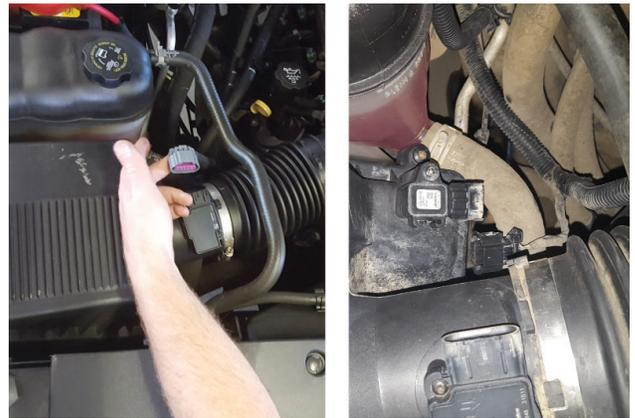
3. Unplug MAF sensor from factory airbox. If applicable, also unplug MAP sensor.
