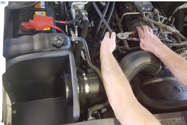
20. Cut fuel hose to length so it can easily connect to hose barb without creating any kinks in its length; then connect it to hose barb.
