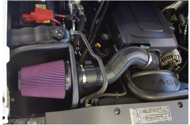
21. Install **cone air filter (1)** into airbox, plug MAF back in and if applicable, plug MAP back in. Use **zip tie (20)** to secure wiring harness, then replace engine cover.
