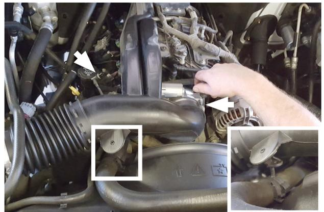
4. Disconnect PCV from resonator chamber, disconnect radiator hose then loosen throttle body clamp.
