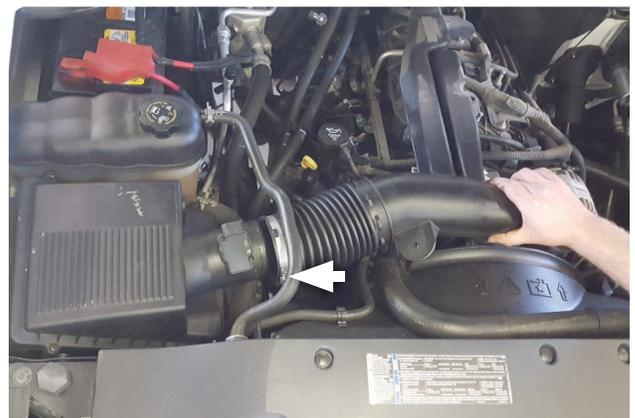
5. Loosen clamp securing intake tube to airbox, then remove it from vehicle.
