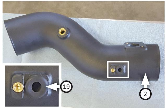
11. Install grommet (19) into intake tube (2).
