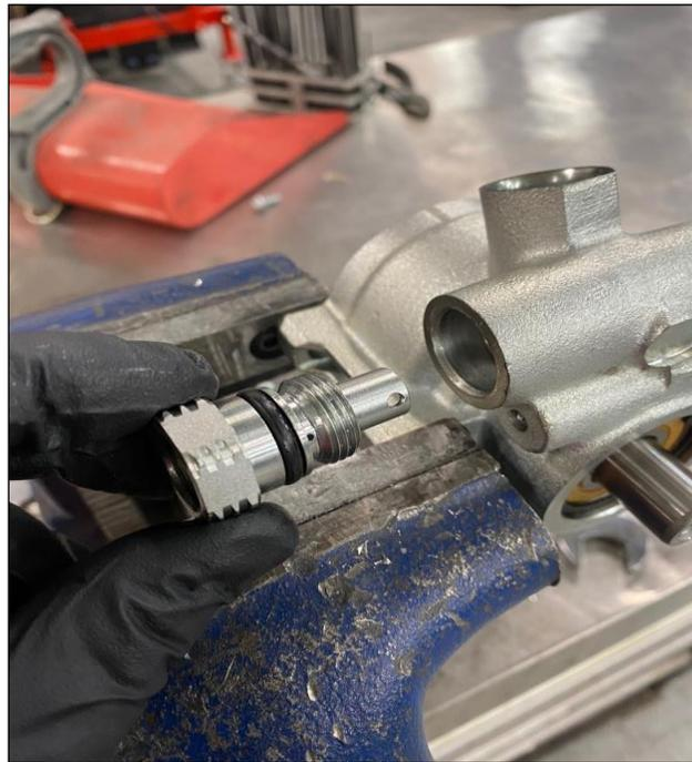
Figure 6 – Flow Control Valve Removal
