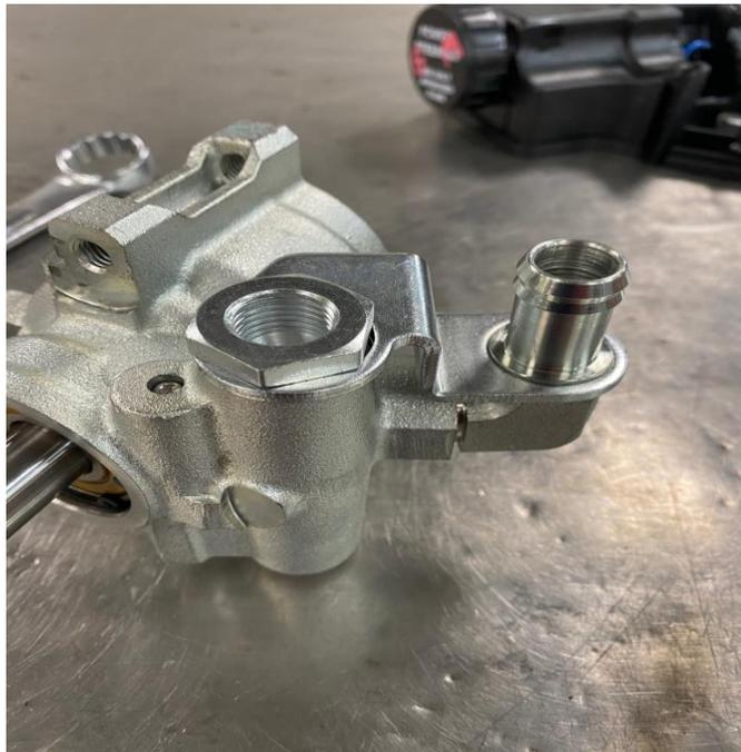
**Figure 8 – Flow Control Valve Installation**
