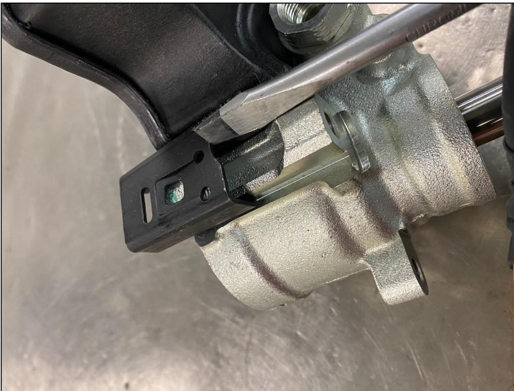
Figure 4 – Retaining Clamp Removal
