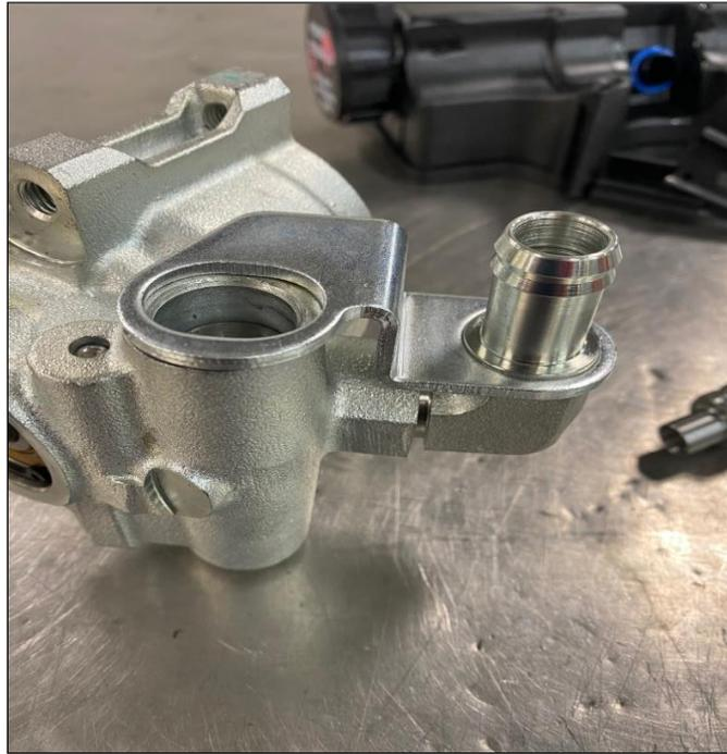
**Figure 7 – Inlet Adapter & Retaining Bracket Installation**
