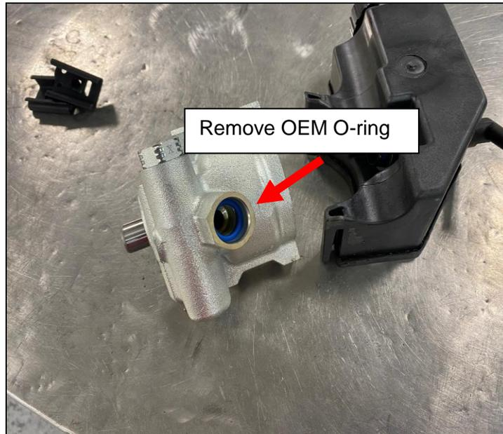
Figure 5 – O-Ring Removal
